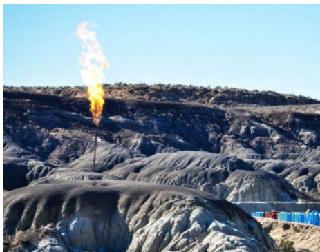
Flaring is a common, yet wasteful, method to get rid of excess methane from oil and gas operations.
